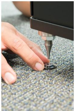
8. Once positioned, adjust the thread depth of the spikes so that the speaker is level and all four spikes are firmly coupled to the floor without any wobbling of the speaker. Tighten the nut on the spike upwards firmly to the bottom of the threaded puck to secure the spike in place.
