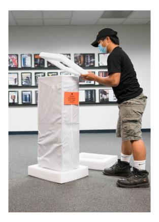
4. As one person tips the speaker back in its foam cradle, pull the protective bag out from under the speaker. Repeat by tilting forward and doing the same to the back. Remove the protective bag.
